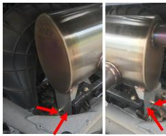
Step 3: Install and mount the Slip-on exhaust with the bolts loosely installed then hook up all four springs. Keep the bolts loose until the rear fascia is reinstalled.
