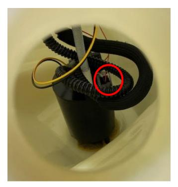
Step 9: Install the new tank into the car, make sure all hoses can move freely. Install the filler neck back onto the tank, this will help hold the tank into place while fastening the straps. Fasten the tank straps until the straps touch the support bar. Reconnect the fuel line, power supply and breather vent. Install the supplied hose clamp onto the breather vent if loose.
