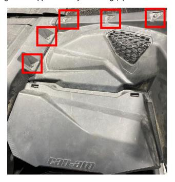
Step 3: Remove passenger side of center council, underneath the glove box and glove box. Total of (8) push darts (two in the bottom of the glove box) and (6) T-30 screws.
