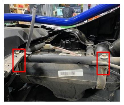
**Step 6:** Now the tank is ready to be removed, slip the filler neck hose off the tank and drop the tank out of the dash. Once removed, blow the old tank off with compressed air.
