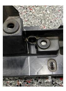
**Step 7:** You will only reuse the air intake/coolant reservoir portion of the shroud. Re install this piece using the OEM mount behind the drivers seat and firewall.
