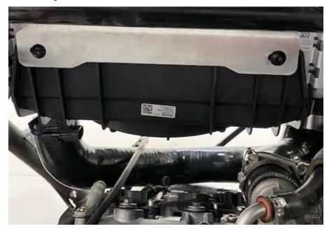
Step 6: At this point you can either run the stock air box, EVP High Flow Intake, or EVP XR Series High Flow Intake. For running the stock air box or EVP High Flow Intake, the OEM plastic shroud will need to be cut. See below (Red Lines). For EVP High Flow Intake Instructions please find them on our website.
