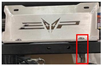
**Step 4:** Install your intercooler using the supplied (4) Torx Screws. It is easier to have your silicone attached loosely to the turbocharger and throttle body.
