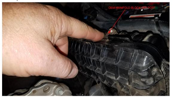
**Step 4:** Move the O-ring from the OEM block off port to the EVP supplied port and install into manifold in place of the block off.
