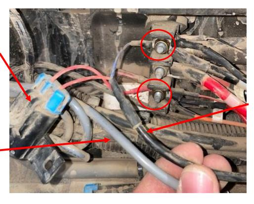
Black power cable with inline fuse. Connect to bus bar.
