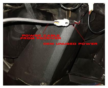
Step 3: Make cable and antenna connections to the receiver box.
