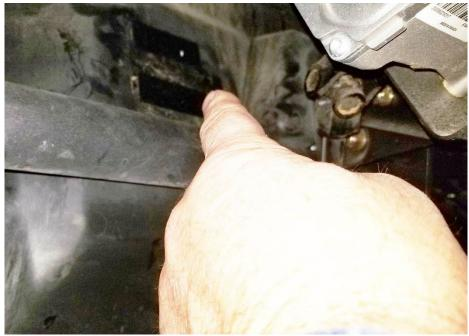
Step 5: Zip tie power cable so it will not interfere with steering or braking functions Step 6: Route cable to the exhaust valve actuator along the inside of the vehicle frame, then to the actuator.
