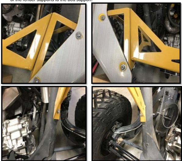
Step 9: Use the 1/4 x 3/4" screws (4) lock nuts (4) and washers (4) loosely install the left and right rear fender support brackets the brake light and body.
