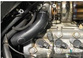
**Step 4:** Install the new silicone onto the throttle body and turbocharger. Use supplied T-bolt clamps to secure.
