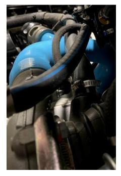
**Step 5:** Install the blow off valve into the charge tube, install the pre filter and clamp down with supplied hardware. If you don't want to run a BOV, install the billet plug into the charge tube and clamp down.
