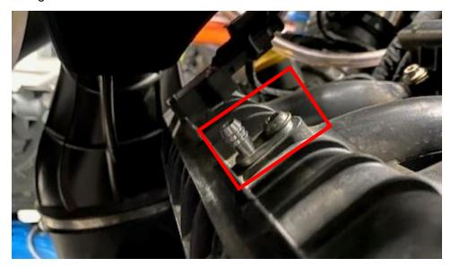
**Step 7:** Install the vacuum line to the BOV and billet adaptor on the plenum. Use a pinch clamp or zip tie to secure.
