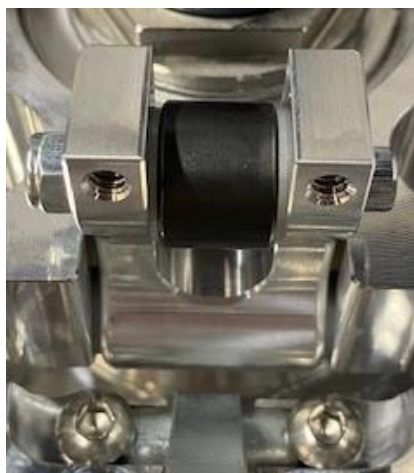
Using Socket Head Screw 1.50" doesn't allow for added weight.
