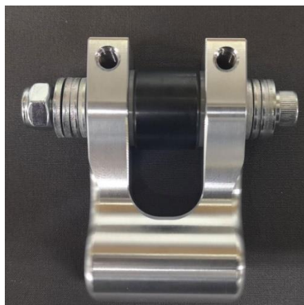
Using Socket Head Screw 2.00" allows for a max of 8 washers adding 10.3 grams.
