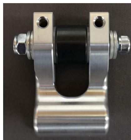
Using Socket Head Screw 1.75" allows for a max of 4 washers adding 5.8 grams.
