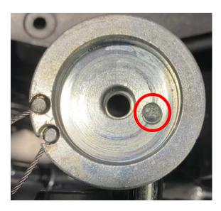
**Step 6:** Install supplied shift lever with supplied set screw. Reinstall the spring, plastic cover and bolt. Make sure the shift lever cut out is facing the passenger side. This will orientate the shift knob in the correct direction.
