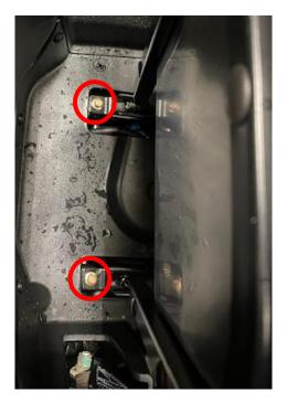
**Step 2:** With a push dart tool remove (11) push darts holding the center console in. Also remove (4) more push darts on both driver and passenger side. This will help remove the center console.
