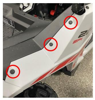
Step 2: Install the correct number plate per side. Reinstall (3) OEM push darts.
