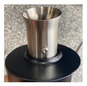
**Step 4:** Install the muffler to the new mid pipe. Install supplied (2) springs holding the muffler to mid pipe.
