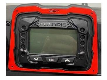
**Step 2:** With a 7/64" drill bit, drill a hole through the plastic dash and insert an Allen screw. Do this for the other (3) mounting holes.
