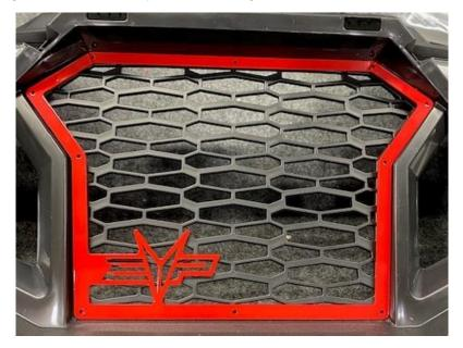
**Step 6:** With a 1/16" Allen wrench and 1/4" socket, fasten down all hardware. DO not over tighten.
