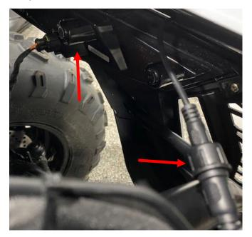
**Step 4:** Remove (4) T-40 screws holding the front clip onto the vehicle. (2) are located in the front of the vehicle under the headlights. The other (2) are located underneath the car where the A-arms connect to the frame. Now remove the front clip.
