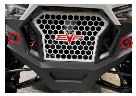
**Step 4:** Install the bumper support behind the front clip, make sure the bend goes underneath the brake block. Reinstall the OEM hardware.
