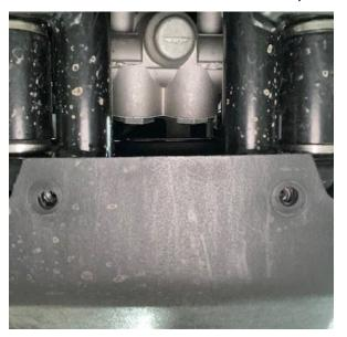
**Step 6:** Install the bumper onto the car. Reuse the bottom two screws to mount the bumper to the frame. Use (2) supplied bolts and washers to mount the bumper to the support in the front of the car.
