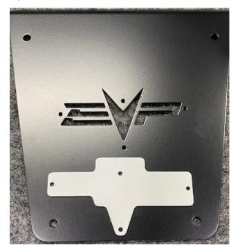
Step 2: Install the lower plate to the front bumper. Use supplied bevel washers and Allen screws.
