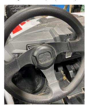
Step 2: Remove the (3) steering wheel screws using a 8mm socket.
