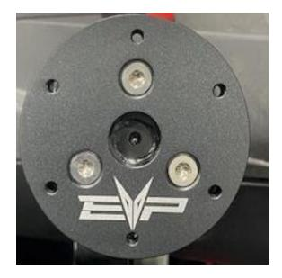
**Step 4:** Install the steering wheel to the adaptor using supplied (6) screws. Use blue Loctite to on threads.
