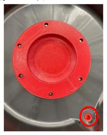
Step 4: With a 1/4" drill bit drill through the shim into the black plastic cover. Place a screw from the inside out. Place a cap nut on the screw from the outside of the cover and hand tighten. Align the shim between each cover support so the nut won't hit. Follow this step for the next (5) holes. Once complete tighten each screw and nut.
