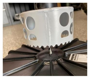
**Step 2:** Once the hole is drilled. Use a file and debur the plastic. Do not use the file aggressively or make the hole size any larger. Once complete use a torch and lightly go around the edges of the hole, making it look shiny.
