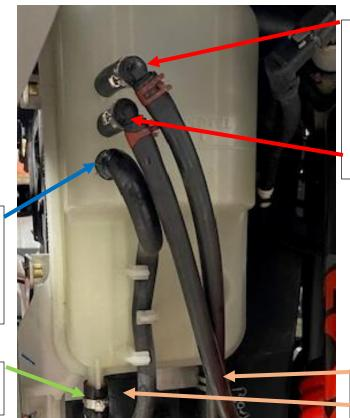
Small radiator hoses. Install a 5/16" 90-degree barb to a 2.0" piece of 5/16" hoses. Mount on the top (2) barbs of the coolant tank.
