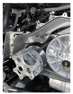
Step 2: Either pull the belt and primary clutch or loosen all (6) M6 primary clutch cover bolts with the primary clutch still in the car. Only take (3) all the way out. NOTE: Apply pressure to the primary clutch cover when removing the last (3) bolts.
