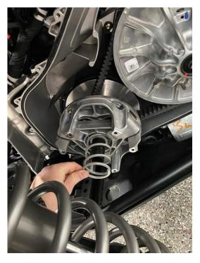
Step 4: Reuse the OEM (6) M6 bolts to mount the primary clutch cover.
