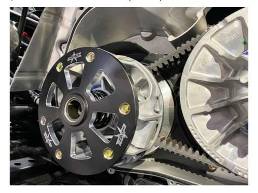
**Step 5:** Install the primary and secondary outer cover.
