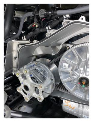
**Step 2:** Loosen all (6) M6 primary clutch cover bolts. Only take (3) all the way out. **NOTE:** Apply pressure to the primary clutch cover when removing the last (3) bolts.
