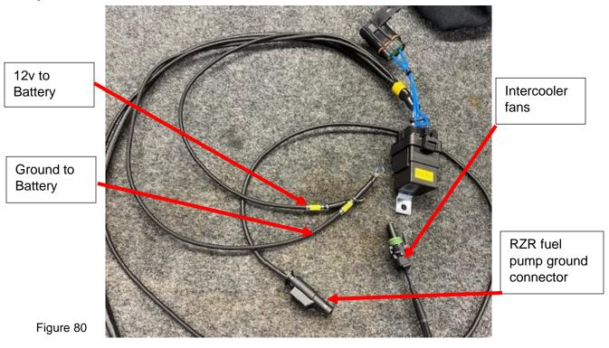
**Step 2:** Locate the fuse block underneath the center tunnel. Below the glove box. Mount the relay to a push dart. Run the ground wire to the frame or battery. Connect the positive terminal
