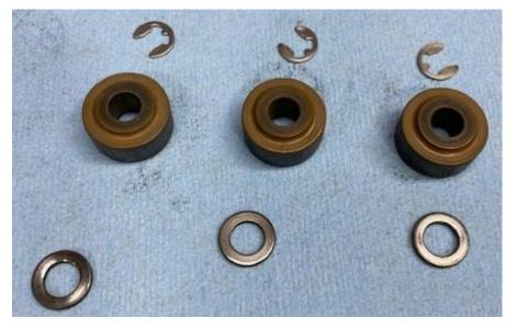
**Step 8:** Reinstall thrust washer, new roller (make sure the indent is on the outside of the roller, against the thrust washer. Install circlip. Make sure rollers can freely spin.
