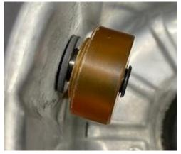
**Step 9:** Re connect both sheaves, making sure helix is riding on all (3) rollers. Reinstall secondary clutch with correct washers and bolt. Torque down to 55 ft lbs. Reinstall CVT drive belt and outer clutch cover.
