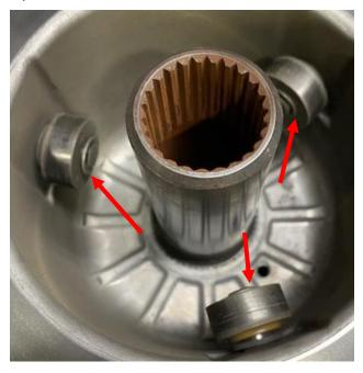
Step 6: Once circlip is removed, slide the roller and circlip off the axle.
