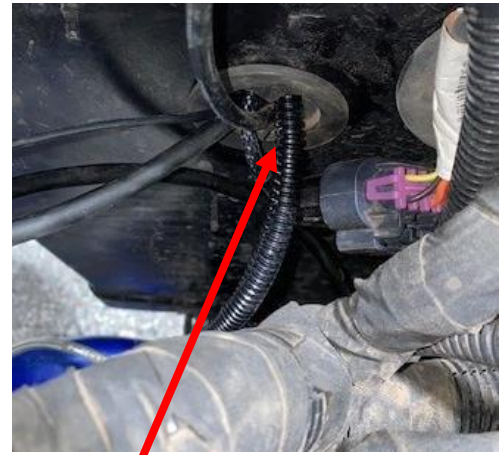
Figure 7, AFR Cable ran through the firewall into the cab.
