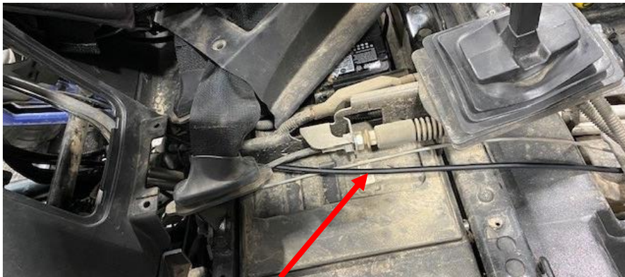
Figure 6, AFR Cable ran down the center console.
