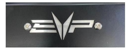
**Step 2:** With a T50 socket remove the (2) screws holding the rear facia to the frame. Keep the plastic step washers.
