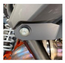
**Step 4:** Install the remaining hardware through the OEM plastic tabs. Place a washer on the head and nut side. Fasten down. Also finish fastening the T50 screws.
