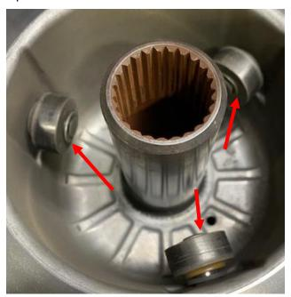
**Step 6:** Once circlip is removed, slide the roller and circlip off the axle.
