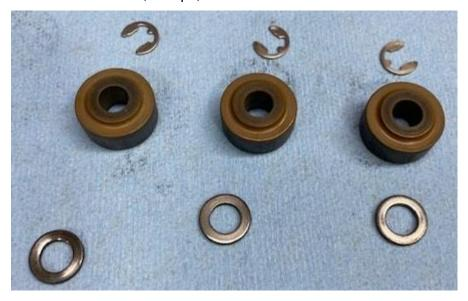
**Step 8:** Reinstall the OEM circlip, be sure not to mar up the new roller. Make sure all rollers spin freely before mating the sheaves back together. Line up the sheaves with your sharpie marks.
