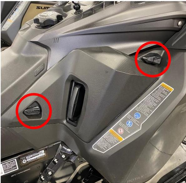
Remove the side panel around the pull cord. Twist both locks upward to unlock.
