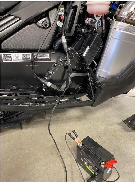
For 2-stroke Models, plug into the OBD port with the 2-stroke Maptuner cable. Then plug the female OBD end of the 2-stroke cable into the BRP Maptuner cable. Connect the terminals to a 12volt battery. The maptuner will turn on.
