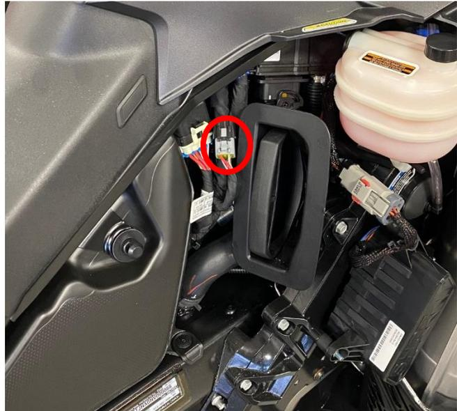
Circled in Red in the OBD port. Unclip the OBD port out of the housing and connect the Maptuner Cable to it.
