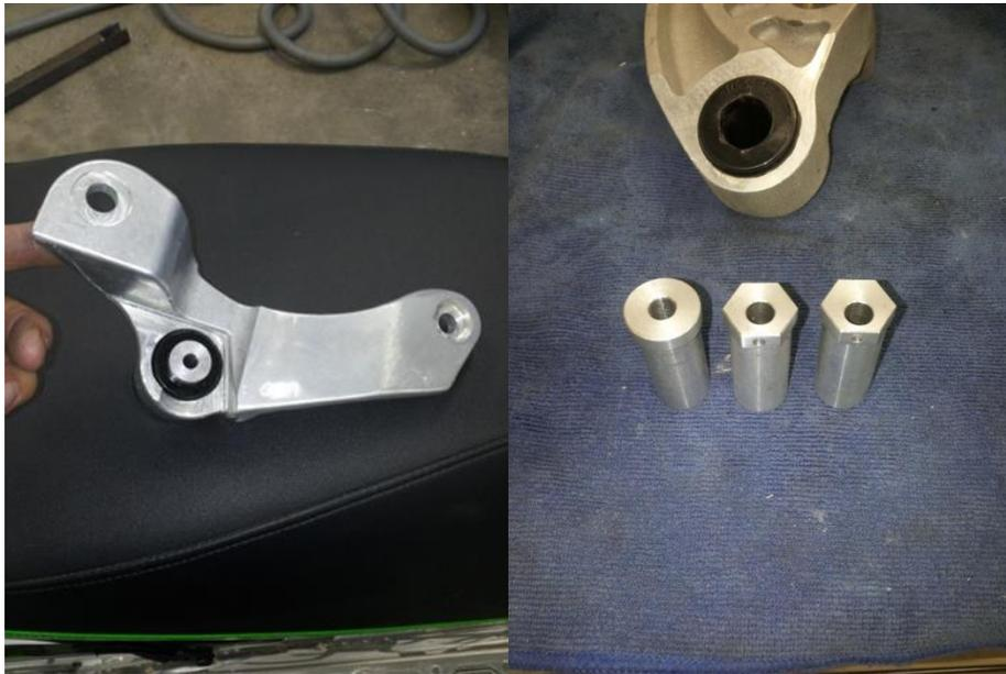
1. Install your new style Turbie/Evo Mag side polyurethane motor mount. Make sure that the polyurethane flange is to the inside and the aluminum flange is to the outside. Some dish soap makes the rubber mount easier to install in the cast aluminum factory engine brackets.
