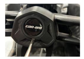
**Step 1 -** Use a flat blade screwdriver to remove the center steering wheel Cover.
