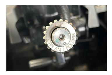
**Step 5 -** Install the coupler nut so the machined surface faces the splined coupler and torque to **66 Ft Lbs. (Polaris) and 44Ft Lbs. (Can Am)**.
