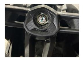
Step 2 - Use a 24mm socket and ratchet to remove the steering wheel nut.
