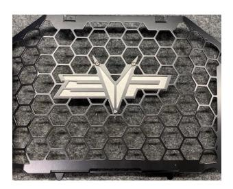
**Step 2:** If replacing just the center grille, unclip the OEM grille from the top two tabs, remove grille. Install the new grille and drill two 5/64" piolet holes and install supplied hardware using a philips screwdriver.
