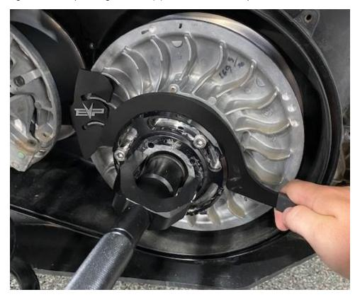
**Step 5:** Remove the helix wrench and secondary holder. Install the belt back onto the clutches. Remove the belt changing tool and spin the secondary a total of 5 times.
