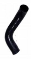
11. INSTALL THE SMALL 1" DIAMETER ELBOW ONTO THE LOWER HOSE BARB OF THE HEAT EXCHANGER (NOTE: THE HOSE MAY HAVE TO BE TRIMMED SLIGHLTY TO BRING IT CLOSER TO THE FRAME AND AWAY FROM THE EXHAUST AND TURBO – DO NOT TRIM THE HEIGHT). USE THE SUPPLIED HOSE CLAMPS TO SECURE THE HOSES.
