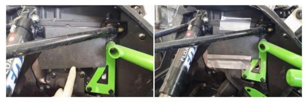
5. USING AN AWL AND HAMMER, MARK THE CENTERS OF THE 4 HOLES
