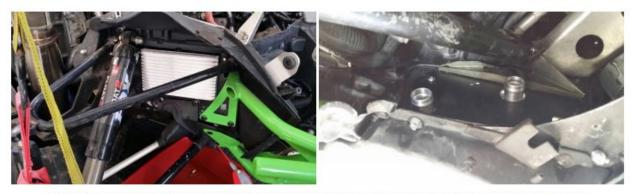
10. INSTALL THE BELOW SILICONE HOSE FROM THE TANK TO THE BACK UPPER HOSE BARB ON THE HEAT EXCHANGER – MAKE SURE THERE ARE NO KINKS (NOTE: THE HOSE MAY NEED TO BE TRIMMED SLIGHTLY)
