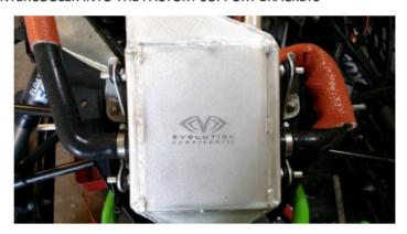
19. IF YOU ARE RUNNING YOUR FACTORY HOOD, YOU WILL NEED TO NOTCH THE SHELL AS SHOWN IN THE NEXT PICTURE. FIT YOUR HOOD CORRECTLY IN THE BACK AND USE THE IN/OUT INTERCOOLER WATER LINES TO MARK WHERE THE NOTCHES WILL BE. MAKE SURE THE NOTCHES ARE ADEQUATE SO THE HOOD WILL NOT RUB ON THE HOSES. DEBUR THE NOTCHES.
