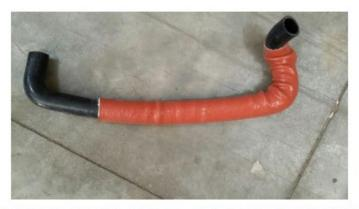
13. INSTALL THE HOSE ONTO THE WATER PUMP INLET AS SHOWN BELOW. THE HOSE WILL CONTACT THE FRAME, SO MAKE SURE THE SLEEVING IS SLID ALL THE WAY DOWN TO THE HOSE CLAMP TO PROTECT IT.
