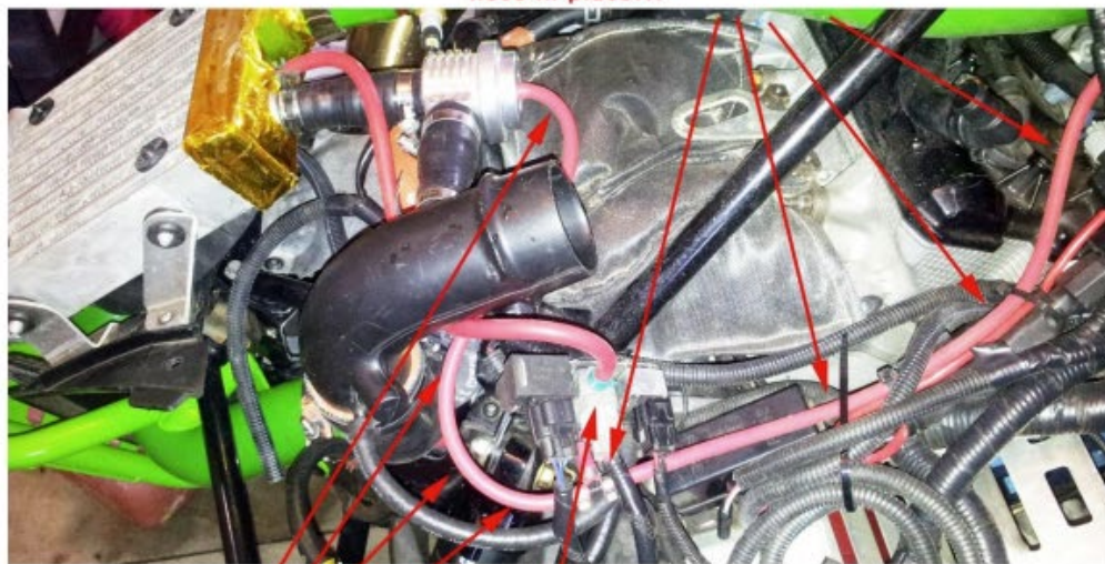
LINE TO BRV BRV Solenoid
