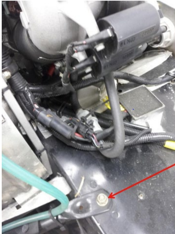
RUNNING BOARD SUPPORT HOOP BOLT
