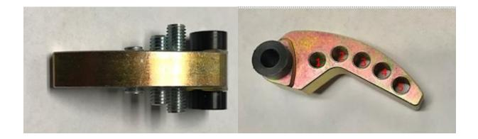
**NOTE:** Always install a set screw on both sides of the weight arm. Install the screws with the provided blue thread locking agent. Make sure the screws are installed with an equal amount of thread engagement.
