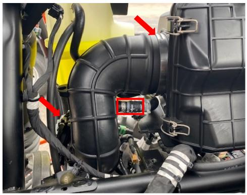
**Step 4:** Remove the OEM intake tube. Remove the valve cover barb from the OEM tube and place it into the EVP silicone tube. Crimp the supplied pinch clamp holding the barb in place. Reuse the two OEM hose clamps.
