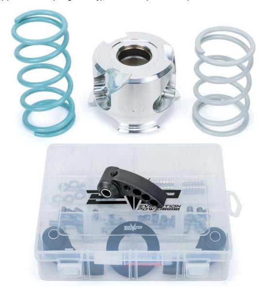
**NOTE**: Always install a set screw on both sides of the weight arm. Install the screws with the provided blue thread locking agent. Make sure the screws are installed with an equal amount of thread engagement.
