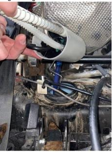
**Step 14:** Slide the rest of the assembly into the tank. Make sure the O-ring is sitting flush on top of the fuel tank. Place fuel pump nut ring on the fuel tank threads and torque to 70 ft/lbs. Verify that the fuel line connections are free of debris. Connect the fuel line onto the pump module. Slide the blue clip towards the driver's side of the vehicle to lock it into place. Re-connect the 4-pin sending unit.
