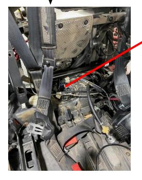
Fuel pump location, and fuel rump ring nut that must be clear of debris.
