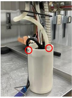
Step 6: Once the pump is released unplug both the Red (+) and Black (-) electrical terminals on the fuel pump. With a razor blade, cut the hose down the ribs of the OEM fuel pump fitting. Do the same on the assembly side. Remove the hose completely and discharge. Remove the pre filter by prying on the plastic ring with a small screwdriver.
