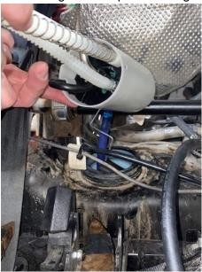
**Step 5:** Once the fuel pump assembly is removed, place it on a clean dry surface. Next step is pushing in the two black tabs on the pump, letting the pump pull out of the white cylinder housing.
