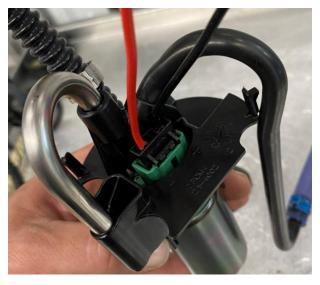
**Step 10:** With a side cutters, cut both terminal ends off the fuel pump assembly. Cut supplied heat shrink in half and slide over both ground and power wires.
