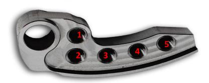
NOTE: Always install a set screw on both sides of the weight arm. Install the screws with the provided blue thread locking agent, making sure the screws are installed with an equal amount of thread engagement.
