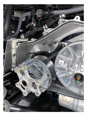
**Step 2:** Either pull the belt and primary clutch or loosen all (6) M6 primary clutch cover bolts with the primary clutch still in the car. Only take (3) all the way out. **NOTE:** Apply pressure to the primary clutch cover when removing the last (3) bolts.
