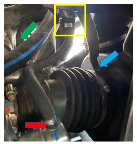
**Step 3:** Remove the worm drive clamp holding the intake tube onto the turbo. (Shown in photo above).
