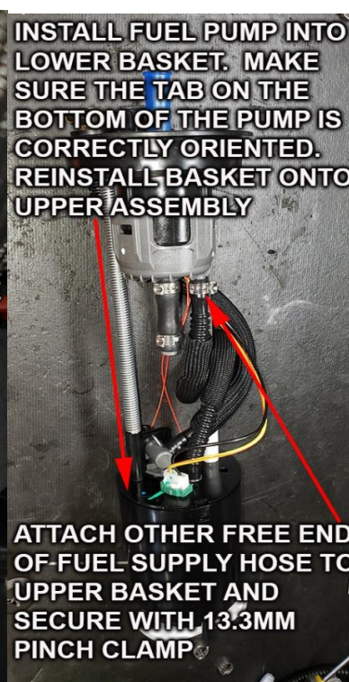
SLIDE INCLUDED 13.3MM PINCH CLAMP ONTO NEW FUEL HOSE. REUSE BRAIDED SLEEVE FROM OLD FUEL LINE. INSTALL FUEL SUPPLY HOSE ONTO NEW FUEL PUMP. PINCH CLAMP AND ROTATE EARS SO IT LOOKS LIKE THE PICTURE
