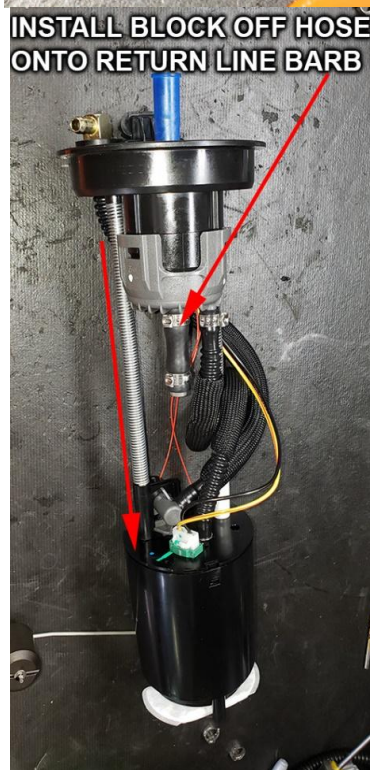
REMOVE FUEL PRESSURE REGULATOR FROM RETURN
