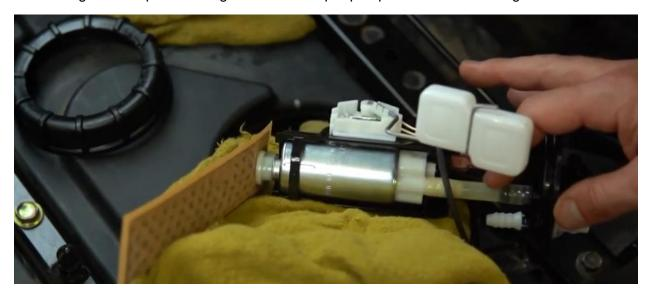
**Step 5:** Once the OEM fuel pump assembly is removed, place it on a clean dry surface. With a flathead screwdriver, remove the OEM pre filter. Also remove both positive (+) and negative (-) terminals off the OEM fuel pump.
