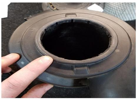
**Step 10:** Once the end cap is removed, use fine grit sandpaper to smooth any ridges and roughen up the surface. Slide the included foam gasket up against the flange of the V Flow Intake – this will seal the area between the V Flow Intake and the OEM filter canister.
