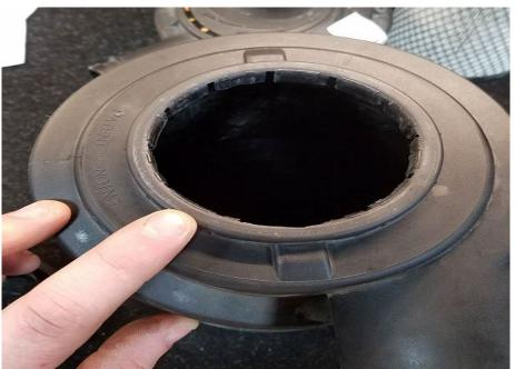
**Step 10:** Once the end cap is removed, use fine grit sandpaper to smooth any ridges and roughen up the surface. Slide the included foam gasket up against the flange of the V Flow Intake – this will seal the area between the V Flow Intake and the OEM filter canister.
