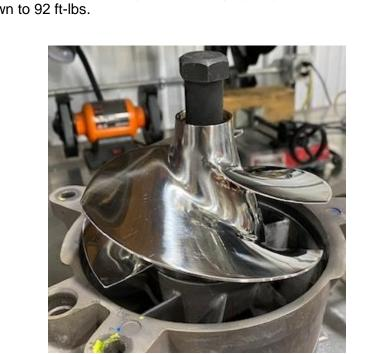
**Step 12:** Install the new impeller and spine onto the jet pump threads. Install the spline tool and torque down to 92 ft-lbs.
