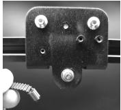
Remove the GT2 belt ends from both sides of the X carriage, but do not remove the belt from the pulleys. Remove X carriage lower bolt, nut and wheel.
