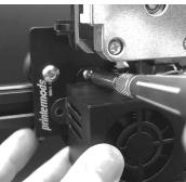
Reconnect the hot end fan shroud, reusing the factory M3 bolts. Be careful not to strain the hot end wiring.
