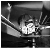
Unplug extruder. Remove the three M3 bolts in the corners of the bracket. Then remove the tensioner arm and the M3 bolt under it.
