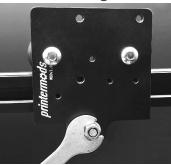
Install the MDD X carriage in the reverse order of removal. Gently tighten the bolts and eccentric nuts until action is smooth and not wobbly. Reattach belts.
