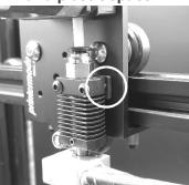
Reuse the lock washers from the factory hot end bolts, and use the supplied M3x20mm bolts to attach the hot end and plastic spacer (in between hot end and x carriage). Insert the PTFE into extruder.
