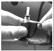
Screw in new Bowden coupler to heat sink, leaving 1 turn unscrewed. Push PTFE down firmly until flat against the nozzle, then tighten.
