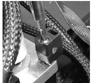
Use the supplied M3x25mm bolt, secure the zip tie anchor to the Z motor. Zip tie securely to the anchor.
