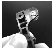
Plastic tensioner arms may crack over time, reducing the amount of tension on the drive gear. Cracked tensioners should be replaced.
