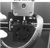
The hot end wiring must be routed in front of the LEFT SIDE Z rail (when viewed from the front). See completed install photos for reference.
