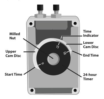
In the above example, the current time is 3:00pm. The number 15 on the 24-hour timer points to the current time indicator.
