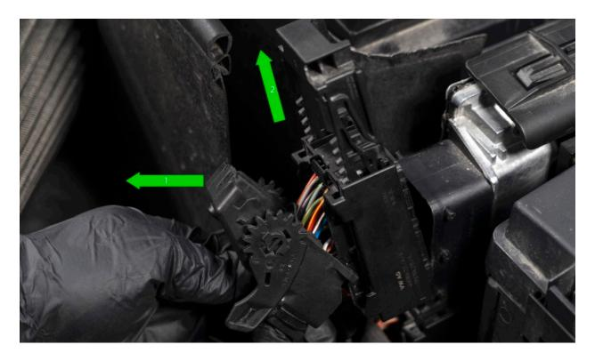
Locate pin #71 and insert de-pinning tool to remove gray dummy pin from connector.
