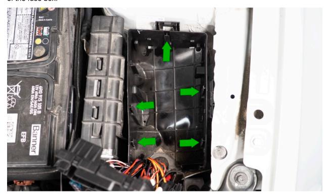
Remove main ECU connector by pulling down on lever located on the front of the connector, which will raise the retaining clip. Once you hear a click, you can pull the connector straight away from the ECU.
