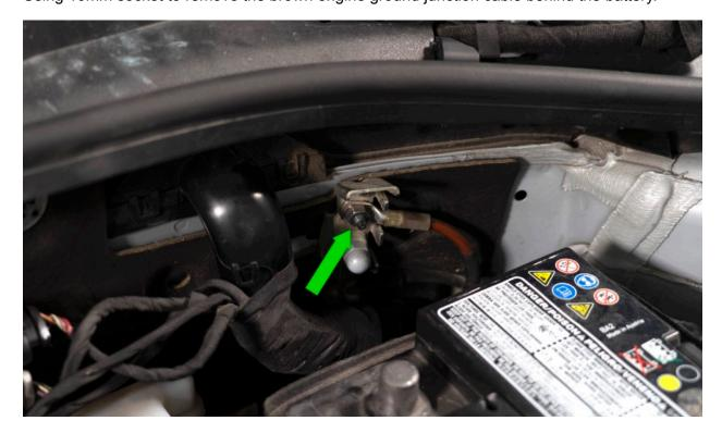
Lay harness on the cowl and install the ground connector onto the ground junction post.
