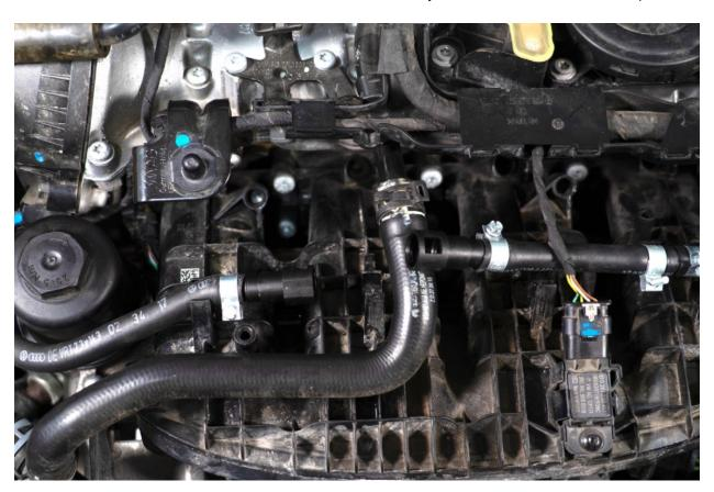
Connect the flex-fuel sensor between the quick connect fittings, then reinstall the fuel line back into fuel line brackets on the manifold.
