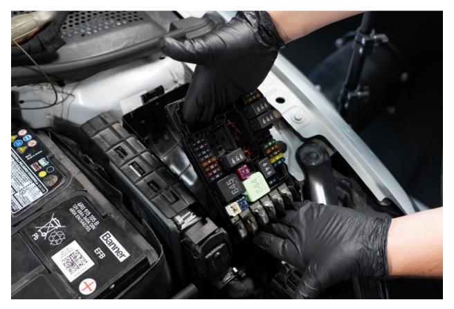
Straighten out harness and allow it to drape over the front of the vehicle. Route the installed ground wire either between battery and ECU, or the ECU and fusebox depending on if you have the metal ECU cover.
