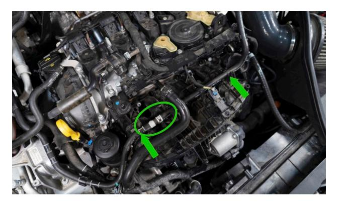
Mark the fuel supply line a quarter inch away from the outside edge of both clamps, then cut the hose on both marks using flat razor or hose cutters. Keep the removed piece for if you decide to ever remove the flex fuel sensor.
