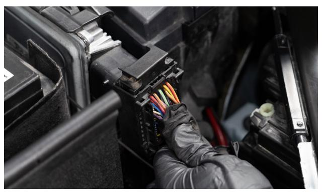
Install back side of ECU connector by inserting guide feet into slots at the bottom of the connector.
