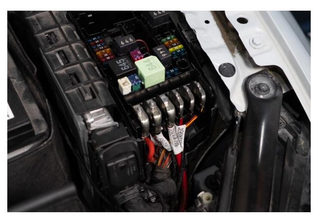
Very carefully push in all 6 tabs using flat head screwdriver, while maintaining constant straight upward pressure to remove top fuse box plate.
