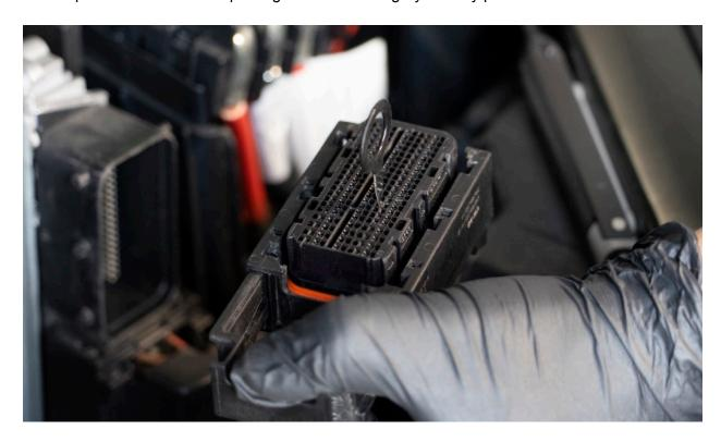
Install ECU pin from Flex Fuel Harness into pin #71 from the back side of the connector until seated. A pick is helpful to help push the pin into its slot completely.
