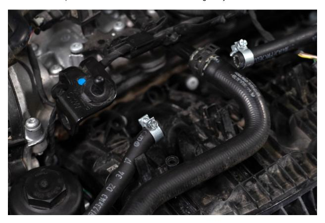
Insert quick connect fittings into each side of the fuel line and tighten hose clamps. Adding small amount of lubrication on the barbs will allow easier install. Be sure to fully seat the fuel hose on each coupler.
