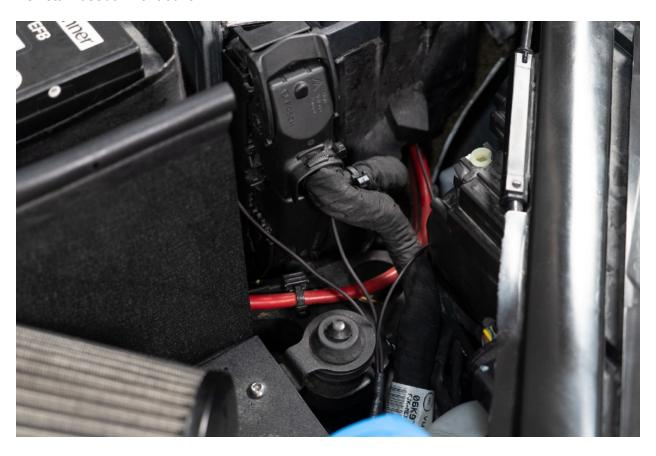
Route Brown Flex Fuel harness underneath the intake and over the intake manifold. This is just our recommended routing. You may have to route a different way for your set up.
