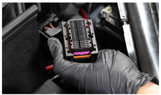
Insert top retaining clip into ECU connector clip and push down fully until seated. then take the back side of ECU connector and insert guide feet into slots at the bottom of the connector.
