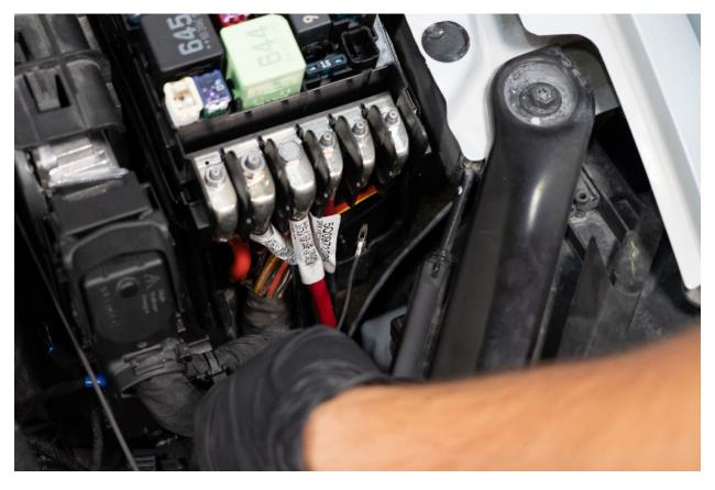
Insert terminal into either of the two blank slots. Assure that you hear a click and give a slight tug to ensure that it is fully seated.
