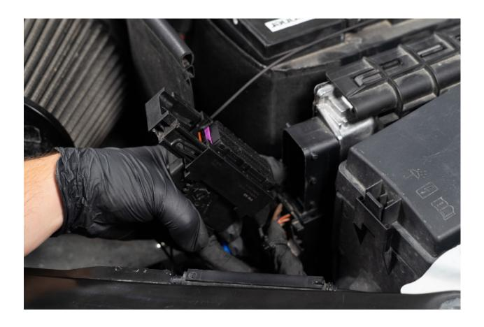
Using flat head screwdriver pick, remove purple retainer clip from ECU harness by pulling straight up.
