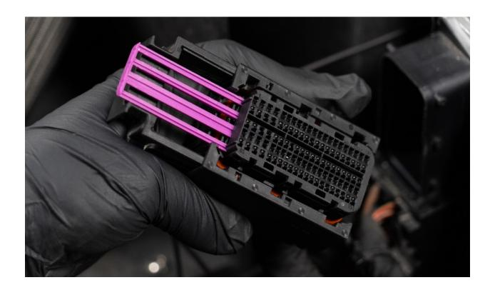
Using flat head screwdriver, split ECU harness and separate the cover from the mounting clip portion of the harness by gently prying upward on the clip.
