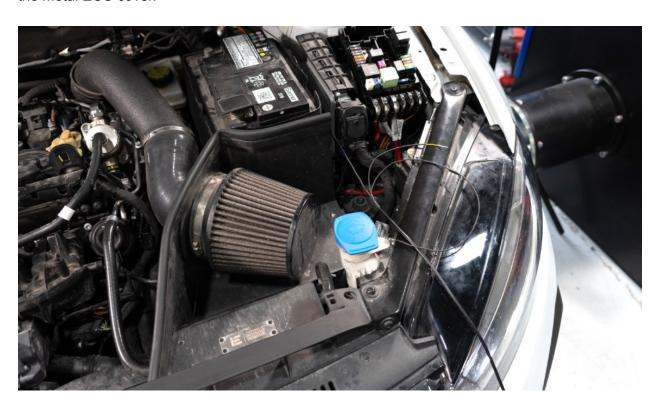
Route the pictured fuse wire underneath the top fuse plate and through gap in fuse box.
