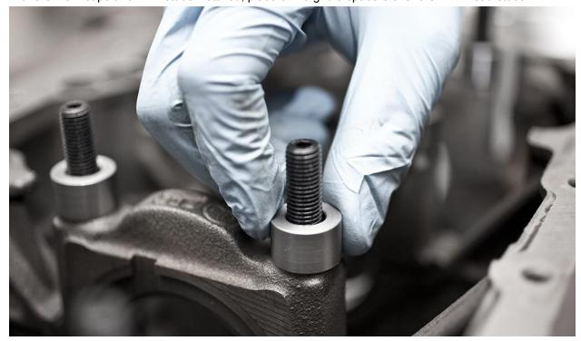
Install the girdle plate over the head studs and spacers onto the block. Make sure the main caps are installed in the proper orientation and fully seated to ensure proper measuring in the following steps.
