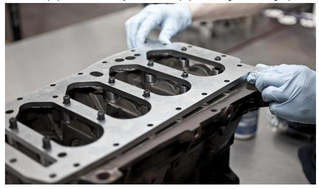
Install the ARP washers and nuts to the head studs with the included ARP assembly lube. Torque to 60ft/lbs using the factory 1.8T torque sequence.
