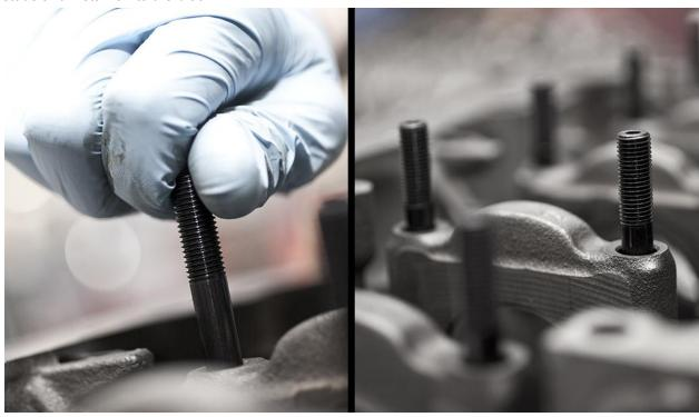
With the main caps and ARP studs installed, place all 10 girdle spacers over the ARP head studs.
