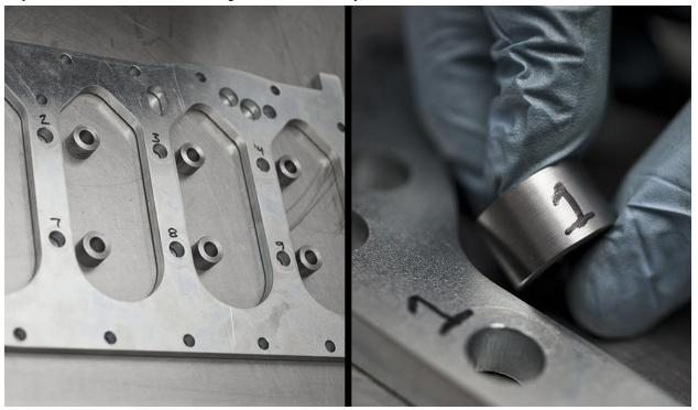
Measure each spacer and subtract your gap measurements to get the final size required. Professionally machine each spacer accordingly to remove excess material and close the gap. The tolerance for the gap between the girdle plate and block is 0.001".
