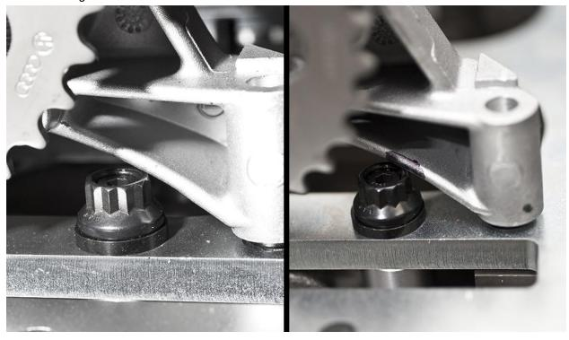
Install the oil pump with the included 60mm bolts and washers. Install your IE extended oil pump chain onto pump sprocket.
