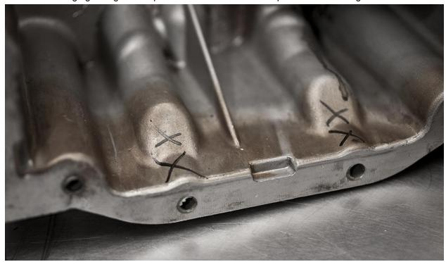
Install the oil pump baffle. Apply a layer of silicone to the block and install the oil pan with the included 35mm bolts and washers. The girdle plate install is now complete and ready for long block assembly.
